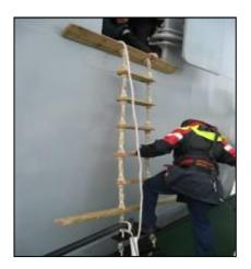
The Pilot should only embark if the top of the ladder is manned. Stepping off the pilot boat onto the ladder requires timing so as to step onto the ladder at the top of a wave
