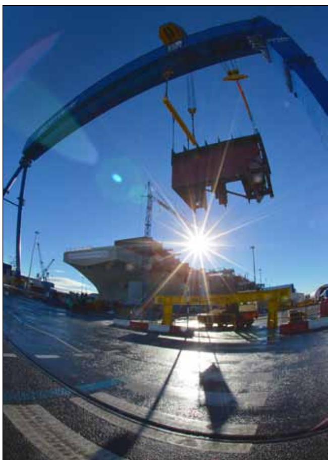
● The Goliath crane picks up the final piece of the ramp ready to lift it into place and (below) hydraulic jacks move one of Queen Elizabeth's rudders into position
