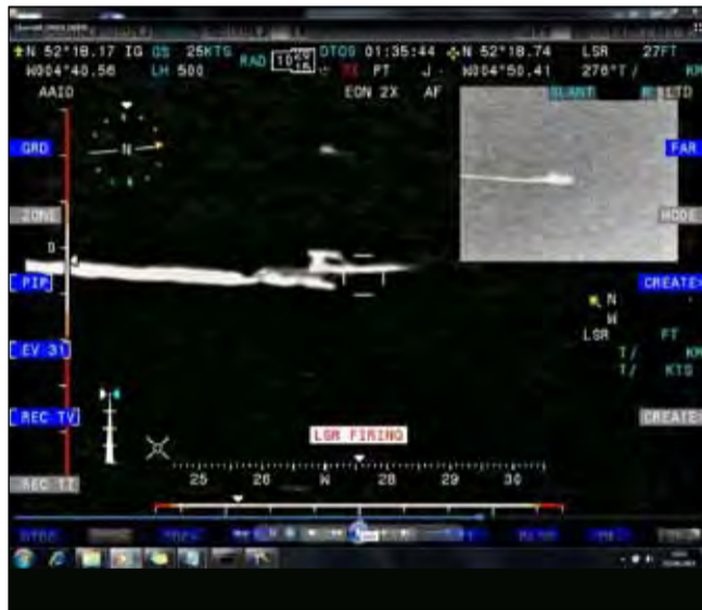
● Above: A small speed boat was lasered by Wildcat's Laser Target Designator
