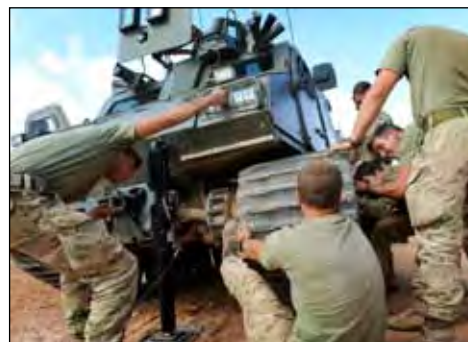
● Mechanics from 40 Cdo perform a track change on a Viking armoured vehicle
