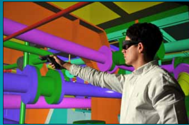
● ...to this – an operator uses an interactive wand to move items of brightly-coloured kit around a virtual engine room. The garish colours come as standard in the off-the-shelf computer-aided design package and make it easier to identify different elements. The engine room of the RN OPVs will not look like this...
