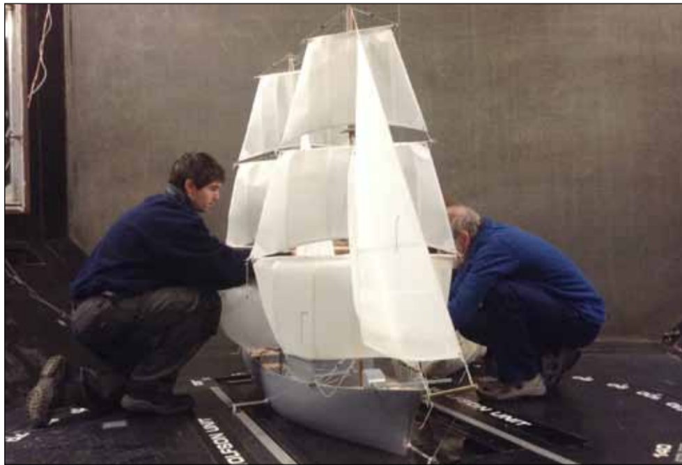
● The scale model of the new Sea Cadet Corps sail training ship is prepared for a test in a wind tunnel
