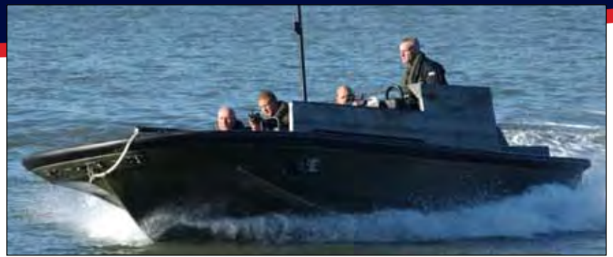
● Instow-designed armour on a Mk3 Rigid Raider (above) and a Land Rover goes through deep water (below)
