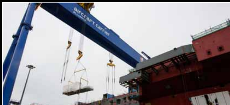
● The gas turbine is hoisted onto the Prince of Wales Pictures: John Linton Photography
