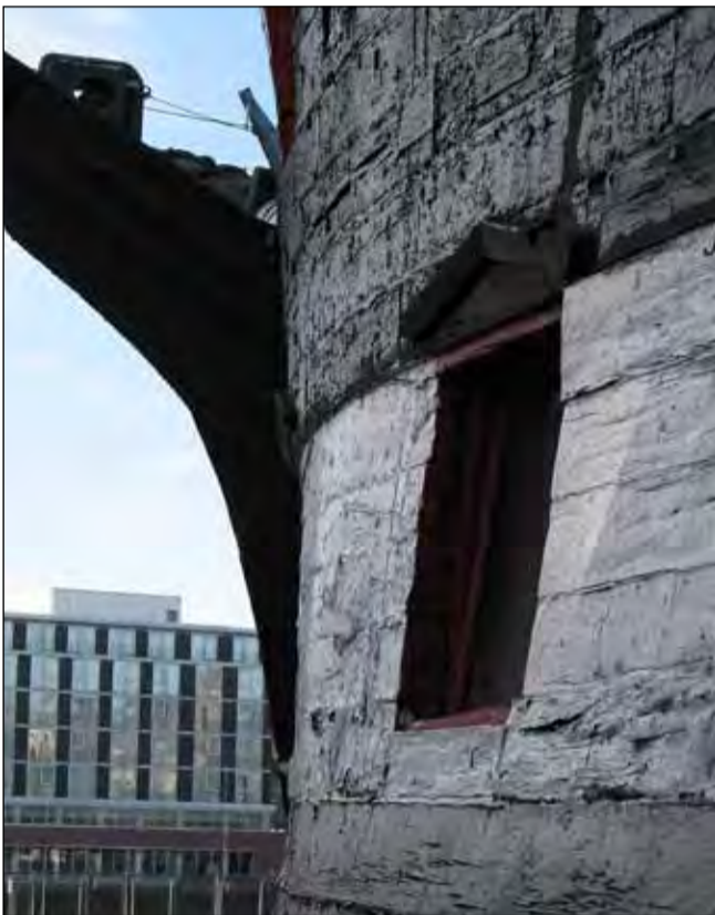
● (Above) The wooden wall of HMS Unicorn – most of her oak hull is original material from the first quarter of the 19th Century, when she was built in Chatham; (left) the unicorn emblem on the prow of the frigate in Dundee; (right) Trincomalee in her Maritime Experience setting in Hartlepool; (below) the decorative transom stern of Trincomalee; (above right) Draught scale marks on a copper gauge the stern of Trincomalee
